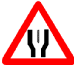
START OF DUAL CARRIAGEWAY
