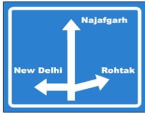
ADVANCE DIRECTION SIGN
