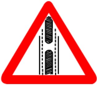
GAP IN MEDIAN
