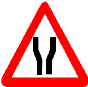
ROAD WIDENS AHEAD
